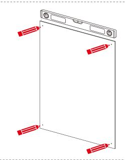
Place the back panel on the wall and mark standoff holes.
